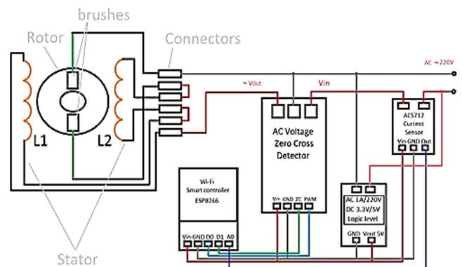
Fig. 6b. Electric motor connection diagram
