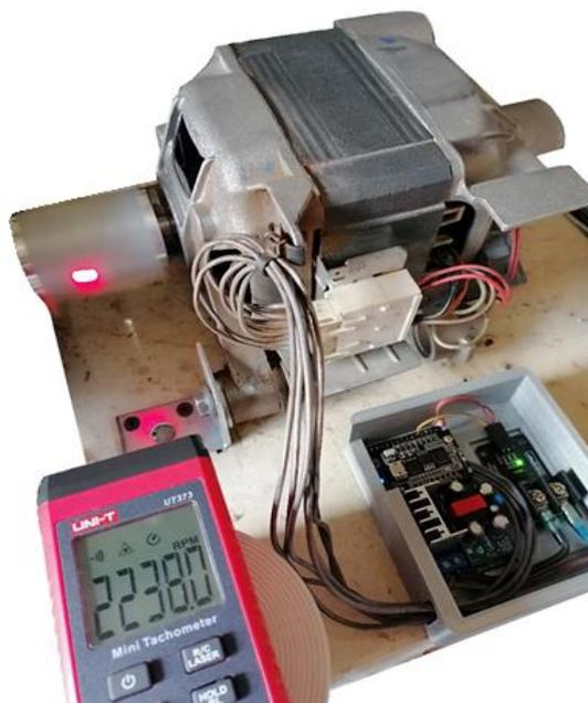
Fig. 10. Laser tachometer for non-contact measurement of revolutions
