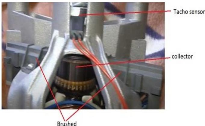
Fig. 4. The location of the collector, the location of the brush holders and the position of the sensor for measuring revolutions
