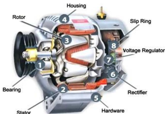
Fig. 1. Alternator components [<https://engineeringlearn.com/alternator-definition-types-working-principle-parts-uses-components-symptoms-of-bad-alternator>]
