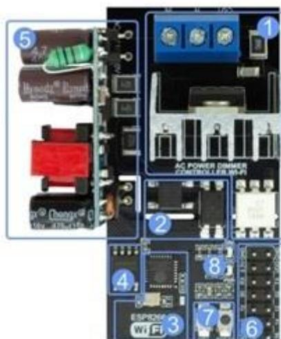
Fig. 7. Collector motor control module [<https://robotdyn.com/ac-dimmer-controller-1channel-ac-esp8266.html>]: 1) AC Dmmer 8A with RC filter; 2) AC Zero-cross detector; 3) WI-FI microcontroller ESP8266; 4) Flash memory 32MB (4MB); 5) AC-DC isolated power supply  $V_{DC} = 3.3V$  (650mA); 6) Pinout 10 I/O header; 7) Buttons: Prog, Reset; 8) LED dimming indicate
