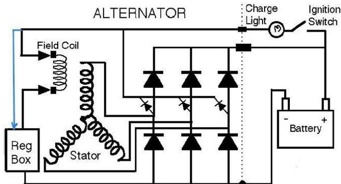
Fig. 2. Wiring diagram of the main components of the alternator [Borysiak, Moore, Sklar, Lamb, Dunn, p.15]
