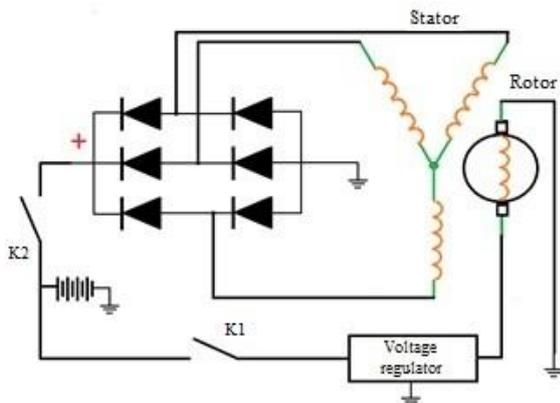
Fig. 6a. Alternator wiring diagram
