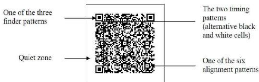
Image 1. The structure of QR code[1]
